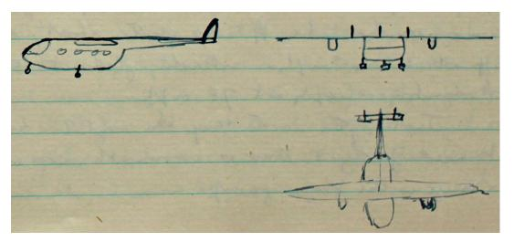
Below the single tail boom, the tail door swings open a vertical post side hinge, enabling a light car or jeep to be driven straight in. The undercarriage is a fixed triangle with steerable nose wheel & air brakes.
